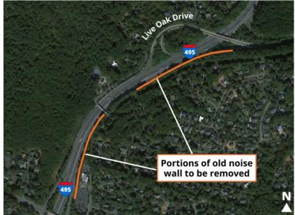
Some noise wall removal activities will occur during overnight hours for safety reasons. With certain stretches of old noise wall located adjacent to I-495, multiple lanes of the Beltway must be closed to enable safe removal. Cranes will lift and stack the old noise wall panels, and then the panels will be transported off-site. Please note that schedules could change if the weather is bad.
